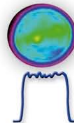
“Top Hat” energy distribution SoLuTis
